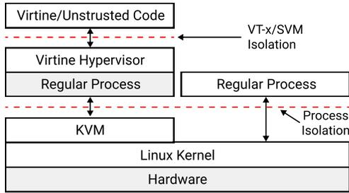
**Figure 1.** How virtines fit into the software stack.
