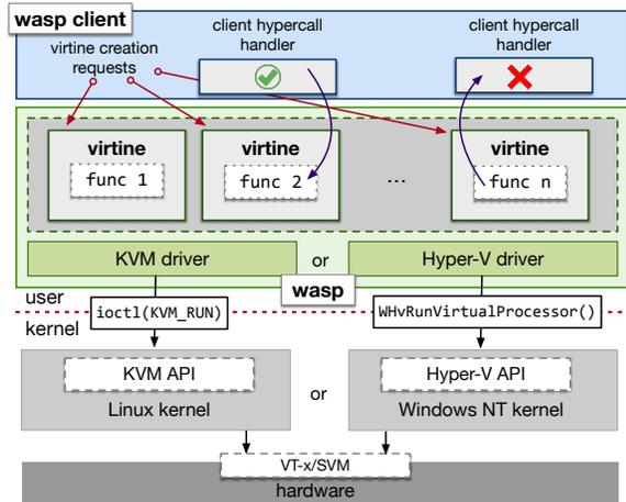
Figure 5. High-level overview of Wasp.
